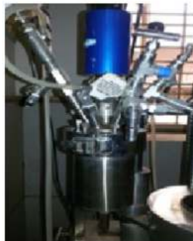
Fig.2: Reactor joint by split clamp bolt
