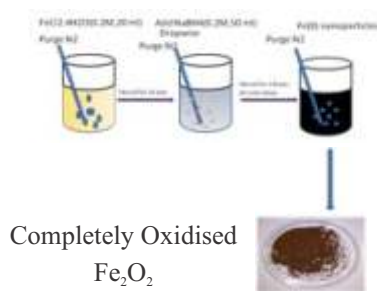
Fig1: Schematic representation of synthesis of iron nanoparticles.
